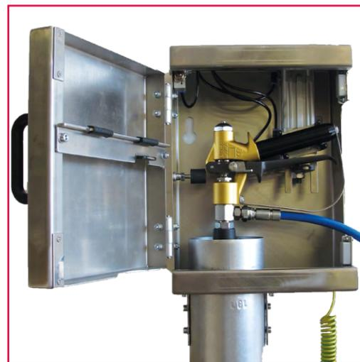
Automates the flushing process for 2K systems. Allows the use of manual spray guns with plural component spray units which automatically flush the gun when the pot life of the mixed material has expired.
