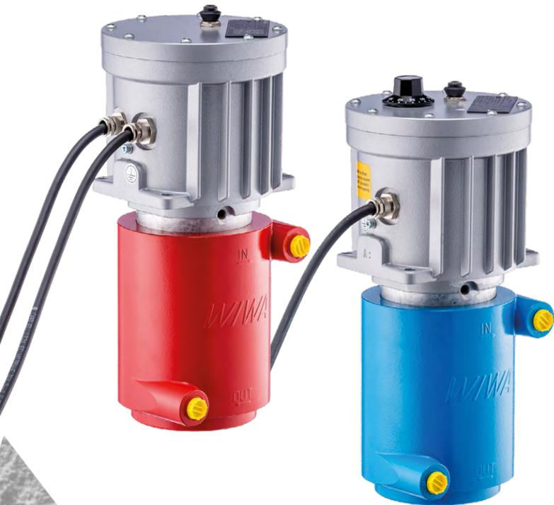
The WIWA material fluid heater with ATEX approval is the optimal addition for cold working environments. It ensures a constant temperature of the injection materials and can bring the container to be processed up to temperature by means of optional circulation. If required, heat can be used to the material to a shorter reaction time and thus accelerate the injection process.
