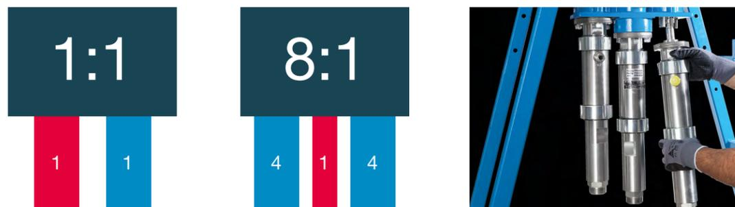
With just a few actions it is possible to modify the system for almost all mixing ratios within a range of 1:1 to 10:1 (also in the decimal range, such as 5.6:1) by exchanging the hardener pump.
