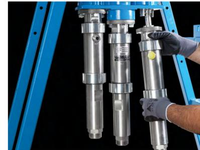
With just a few actions it is possible to modify the system for almost all mixing ratios within a range of 1:1 to 10:1 (also in the decimal range, such as 5.6:1) by exchanging the hardener pump.
